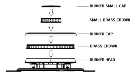
Assembly of the burner caps and burner grates
