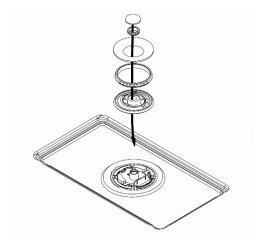
Once in place, you may check the fit by gently sliding the burner cap from side to side to be sure it is centered and firmly seated. When the burner cap lip makes contact inside the center of the burner head you will be able to hear the burner cap click.
